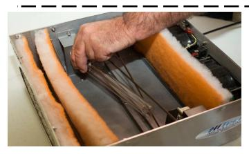
4. Install by holding on the base only. Lean bulb over in the direction of the safety latch on the socket, insert the bulb and then straighten bulb as it inserts into the bulb socket
